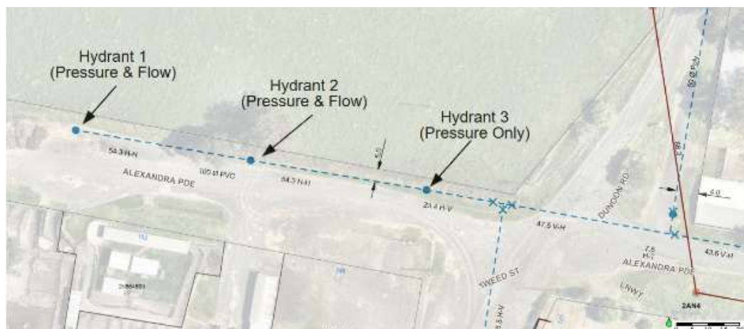
Figure 13: Lismore Council Flow and Pressure Test map of the hydrants used for this test.
